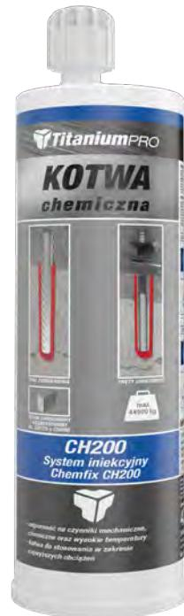
A two-component chemical anchor made of styrene free polyester resin with very high bond strength. Used to fix steel threaded rods and reinforcement rods in the heaviest load applications. The lack of styrene reduces unpleasant odours and vapours that are harmful to human health and the environment. It is highly resistant to mechanical and chemical factors as well as high temperatures.
