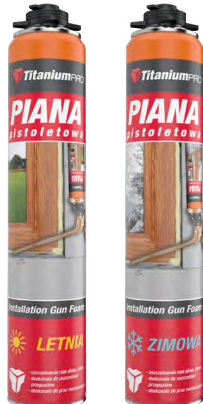
Standard polyurethane foams are characterised by excellent expandability and insulating properties upon curing. They adhere perfectly to most construction materials and substrates. Curing occurs by absorbing moisture from air. In dry environments and lower temperatures with low humidity, moisture should be introduced into the gap. A cured foam is not resistant to UV radiation. It must therefore be protected against such.
