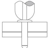
1. The rivet shank is placed in the riveting machine and the rivet head is installed in the hole between the parts to be joined.
