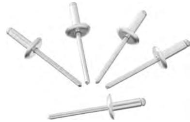
Extended flange rivets are used to fasten thin materials to hard substrates. The large flange also helps mask an oversized hole and prevent free migration of moisture.
