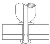
3. Further increase in the breaking force in the riveting machine and pulling of the rivet shank causes a crack formed in a well-defined place.
