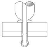
2. The rivet's shank is pulled by the jaws of the riveting machine. This causes deformation of the rivet head situated on the inner area of the elements to be joined.
